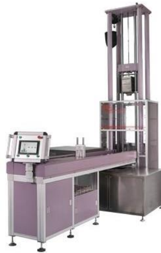
Figure 1-5 Deep Zhen Wan test company DIT shock drop Hammer punch test machine
