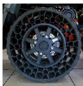
Figure 1-2 honeycomb explosion-proof tire damaged by external force
